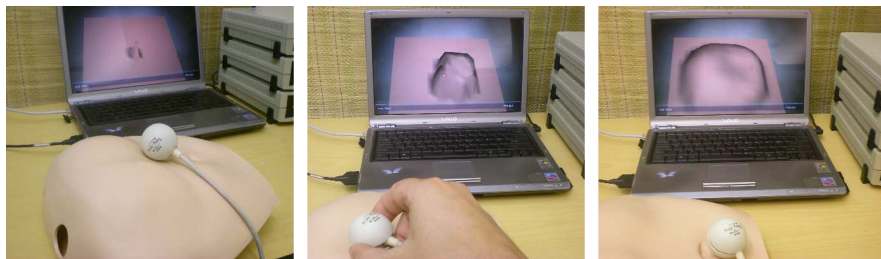
Fig. 12 Scanning SimMan abdomen module: sensor alignment (left), scanning in progress (middle), completed mesh (right) Grid size 40x40 cm, 20x20 points. Scanning time: under 2 minutes.
