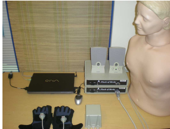
Fig. 5 Touch-augmented Anne Torso manikin, augmented with a tangible user interface. System components: the manikin object, laptop PC, Flock of Birds tracking system, speakers.
