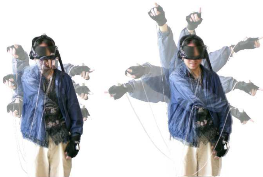
Figure 3: Two composite images showing the extents of the static (left) and sliding views (right). For this test, the user was asked to draw the contours of his visible areas, without turning his head. The view sliding technique more than quadruples the area.
