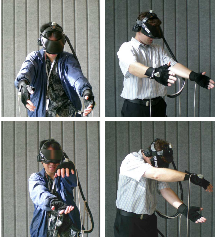
Figure 1: VR users demonstrate areas of hand visibility for a 40° HMD: horizontal (top) and vertical (bottom). Both hands and head are tracked in 6 degrees of freedom. In order to see their hands, users sometimes have to assume very uncomfortable poses (bottom right).
