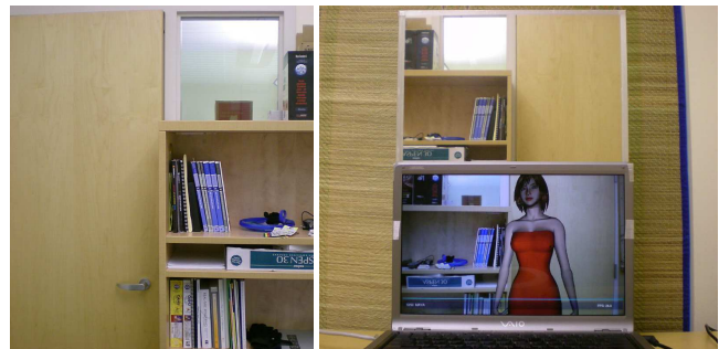
Figure 8: A virtual mirror: adding a virtual character to a real office scene (left). A real mirror is mounted on top of a laptop, providing a reference view. The laptop operates in a virtual mirror mode, showing the same scene, augmented with an animated 3D character.
