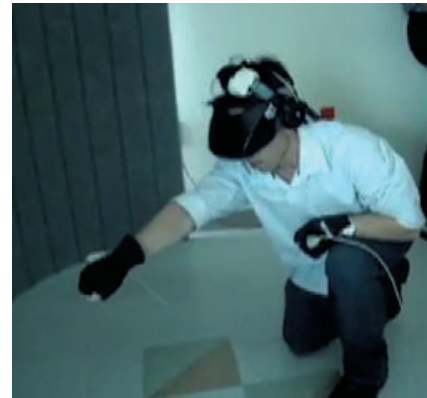
Figure 2. A medical student, wearing a head-mounted display (HMD) and two sensor gloves checks the pulse of a simulated casualty in the virtual environment.
